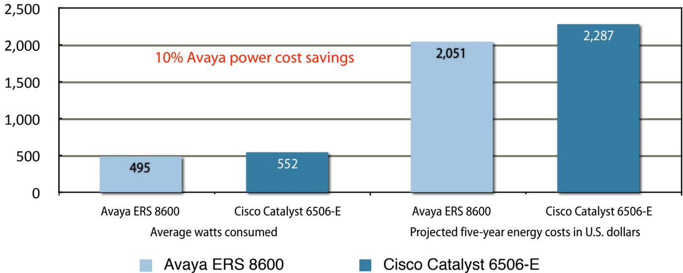
Notes: 120 copper ports (24 Gigabit Ethernet ports and 96 Fast Ethernet ports) were connected. Cost projection is based on the 2006/2007 Average Commercial Electric Price of US\$0.0946 per kilowatt hour.
