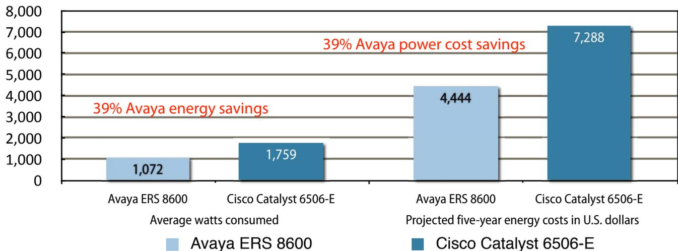
Notes: 96 copper ports (48 Gigabit Ethernet ports and 48 Fast Ethernet ports) were connected. Cost projection is based on the 2006/2007 Average Commercial Electric Price of US\$0.0946 per kilowatt hour.
