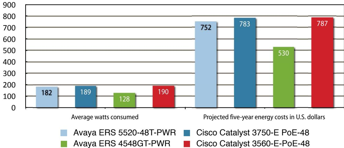
Note: Cost projection is based on the 2006/2007 Average Commercial Electric Price of US\$0.0946 per kilowatt hour.
