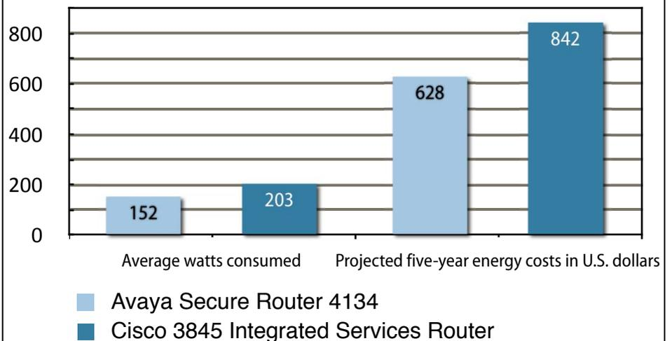
Note: All FE ports active, WAN ports idle. Cost projection is based on the 2006/2007 Average Commercial Electric Price of US\$0.0946 per kilowatt hour.
